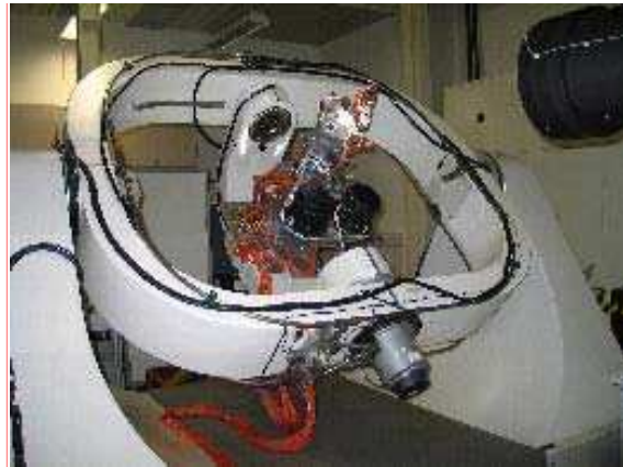
Figure 9: DBT U-Table with 3 redundant Fine Sun Sensor heads & 2 Gyros accommodated
